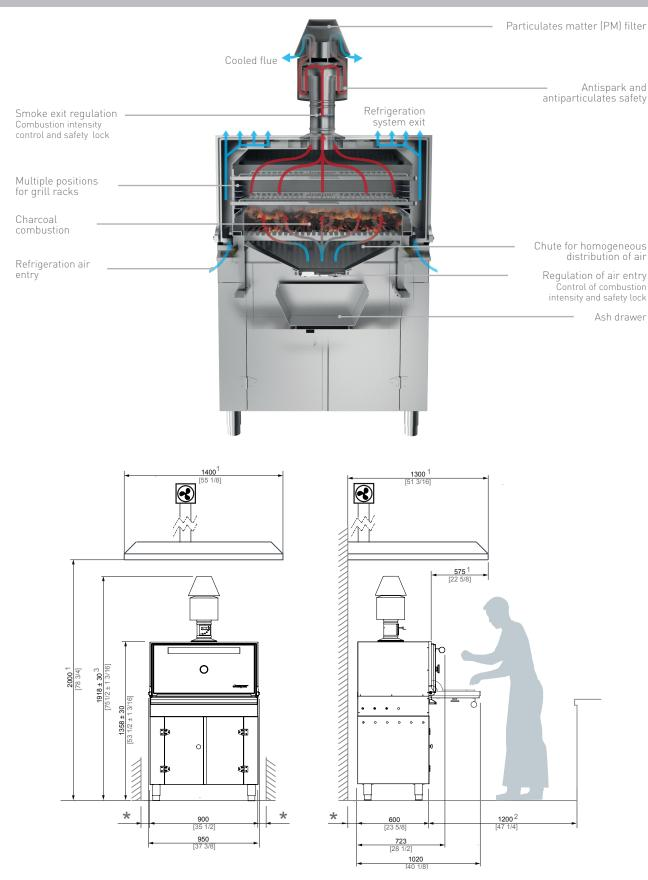
\* MINIMUM DISTANCE TO FLAMMABLE ELEMENTS: 300 mm [12 in] / RECOMMENDED DISTANCE TO ANOTHER ELEMENTS: 100 mm [4 in]
