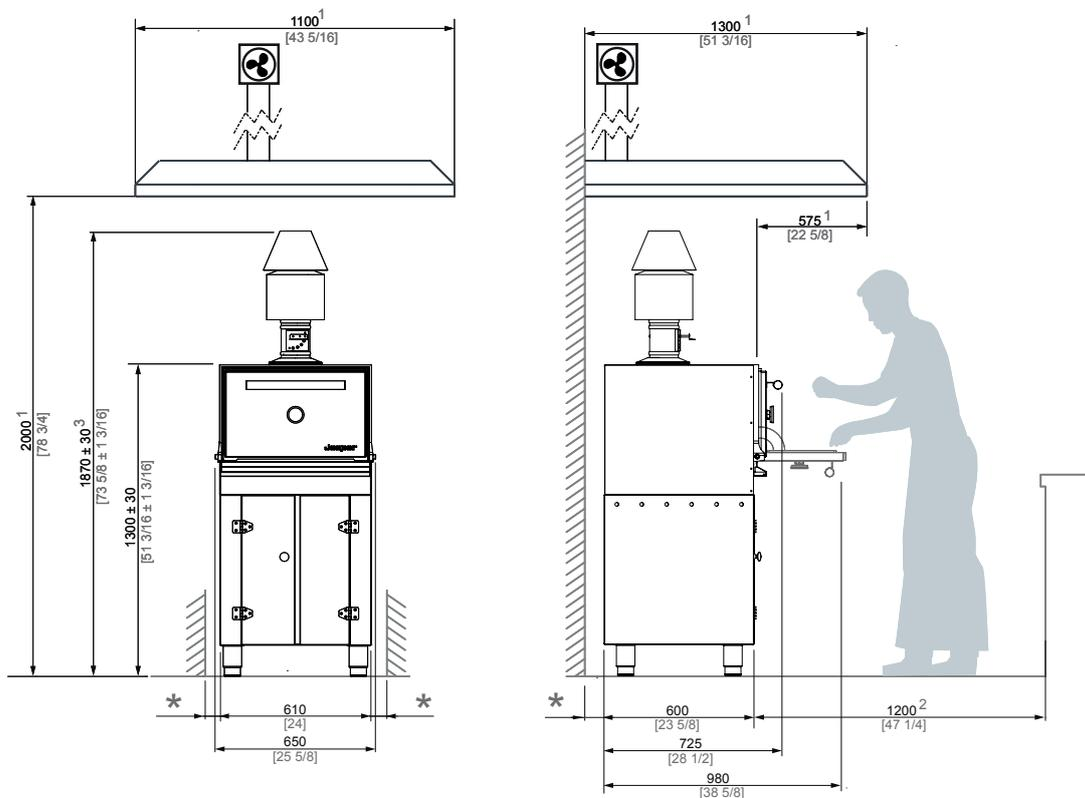
\* MINIMUM DISTANCE TO FLAMMABLE ELEMENTS: 300 mm [12 in] / RECOMMENDED DISTANCE TO ANOTHER ELEMENTS: 100 mm [4 in]
