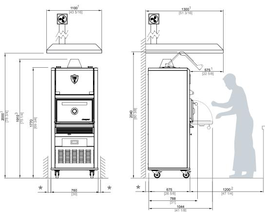
\* MINIMUM DISTANCE TO FLAMMABLE ELEMENTS: 300 mm [12 in] / RECOMMENDED DISTANCE TO ANOTHER ELEMENTS: 100 mm [4 in]
